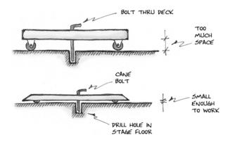
Grinding the end of the pin so that it is slightly pointy will make it easier to insert it into the deck. Never use more than two bolts, because it will be far too hard to line the piece up, and besides, it is just not necessary. If you concentrate on getting one pin into its hole, it is fairly easy to rotate the unit so that the other simply drops in on its own.
